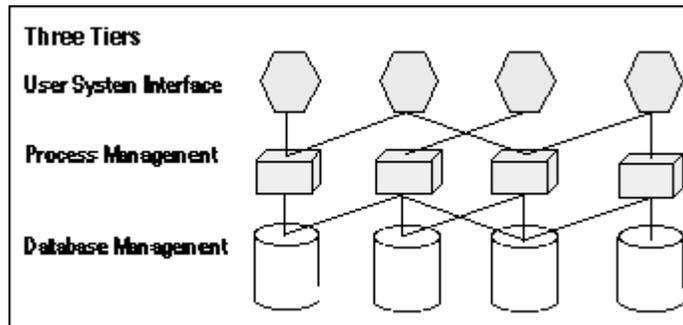
**Fig. 4.19 Three-tier Client/Server Architecture [37]**
