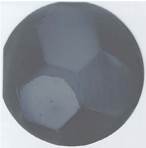
Figure 7. Patterned tungsten film produced by the prototype Programmable CVD reactor.
