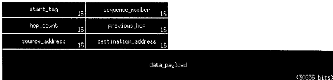
Fig 6. Packet format used for ISS and ground user data transfer
