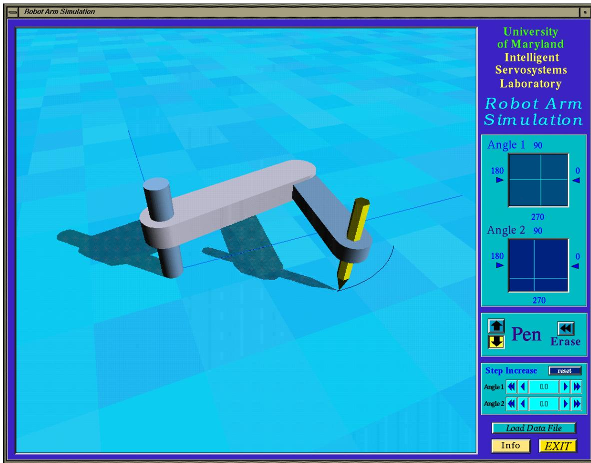
Figure 3: Simulation of Writing Instrument Manipulator.
