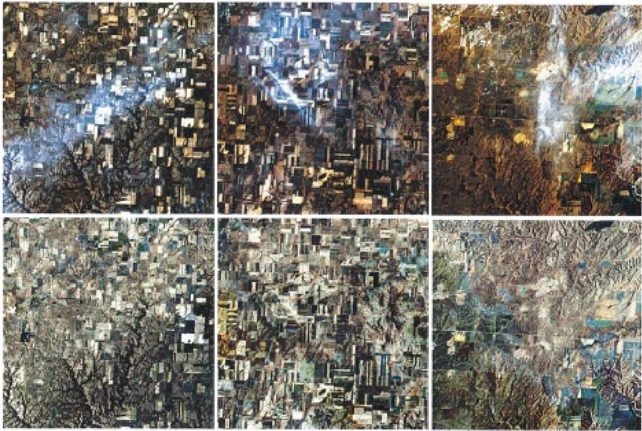
Fig. 6. Atmospheric correction examples of three scenes (Bands 1, 2, and 3). The first row shows the true color composite images before atmospheric correction, and the second row after atmospheric correction.
