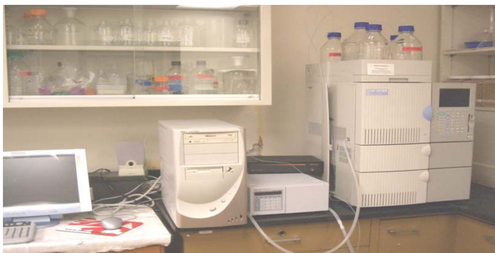
Fig 3.6.1. HPLC system: (left to right) Monitor, Computer with Class VP software and Versa Comm+4. PCI data acquisition board, Shimadzu RID 10A refractive index detector, and Shimadzu LC 2010A HPLC system.
