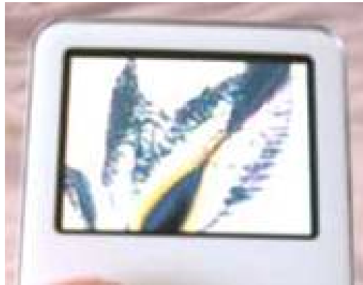
Figure 5.1 Mechanical failure—cracked top glass layer of LCD screen [4]
