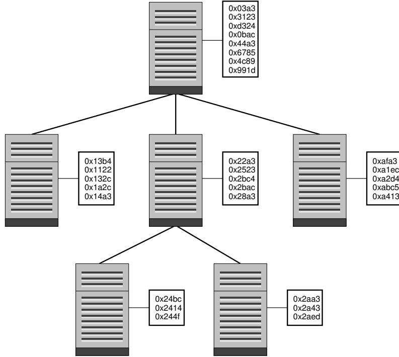
Figure 6.2: An example partition tree for the keyword `Red`.
