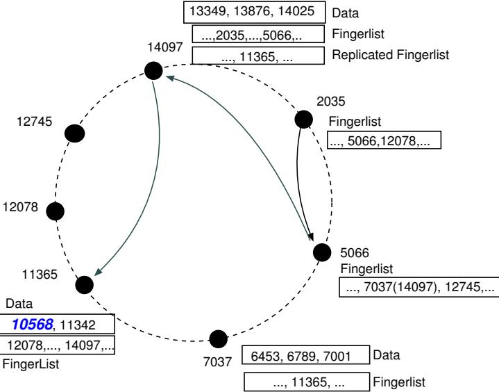
Figure 5.6: LAR routing and replication in Chord
