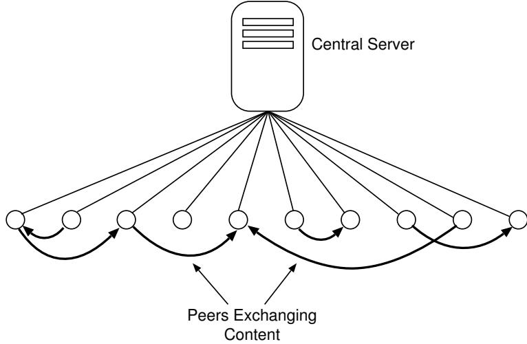
Figure 2.1: Architecture of the Napster file sharing system
