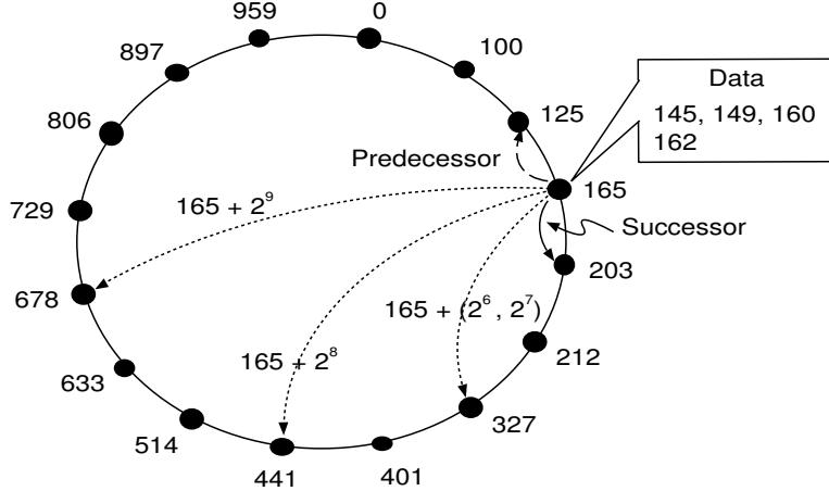
Figure 2.3: The figure shows an example Chord network. Chord is a DHT-based structured P2P system.
