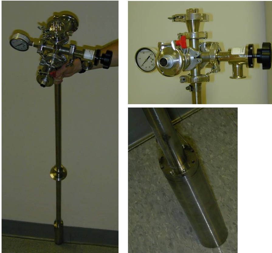
Figure B.3 Clockwise from left: The probe; close up of the top of the probe showing the BNC connectors, pressure gauge and the evacuation valve; The bottom can and that can be screwed on hermetically with an indium seal.
