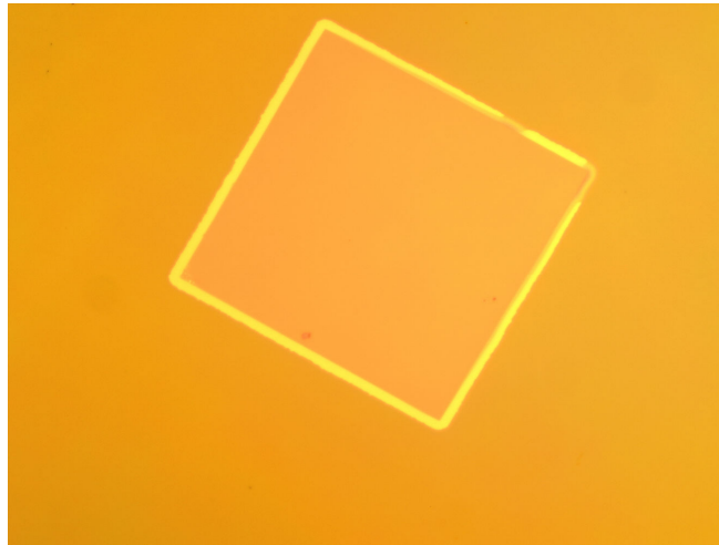
Figure 2.6 Optical picture of a membrane showing undercut of oxide by HF. The undercut is seen as a border
