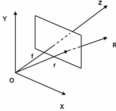
Figure 3.1: Image formation of a pinhole camera.
