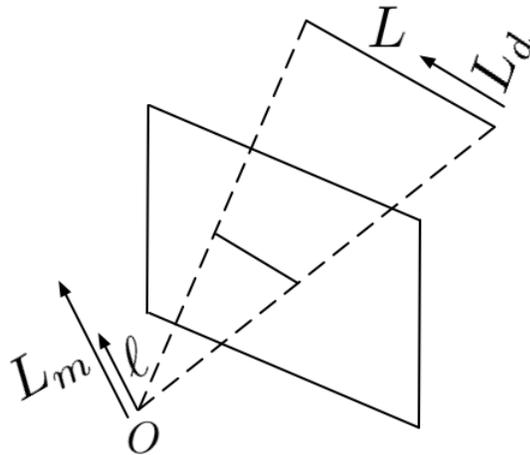
Figure 2.3: Plücker representation of a line  $L$  as  $(L_d, L_m)$  and its image  $\ell$ .
