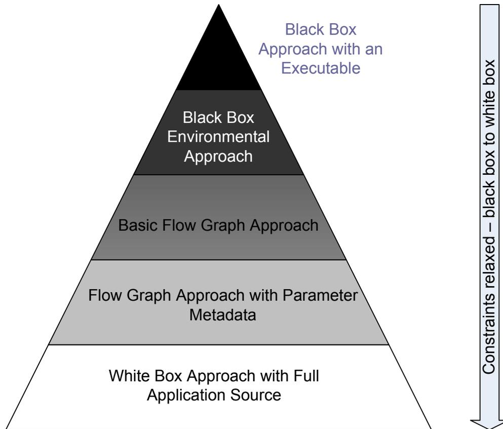
**Figure 7 Black Box to White box - A hierarchy of fault injection based approaches for finding vulnerabilities**
