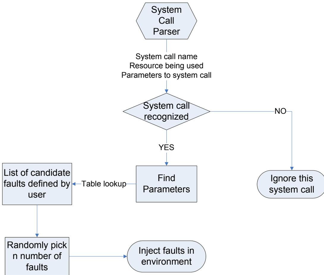
**Figure 2 Fault selection algorithm**
