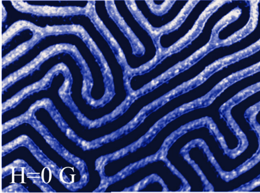
Fig. 2.7 For sensors with out-of-plane magnetization, the stripe structure diffracts the incident light inducing nonlinear response.
