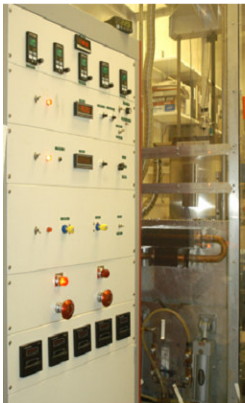
Fig. 3.2 Photograph of the LPE growth furnace and adjacent control panel. Labview software is interfaced to the control panel to coordinate the growth process.
