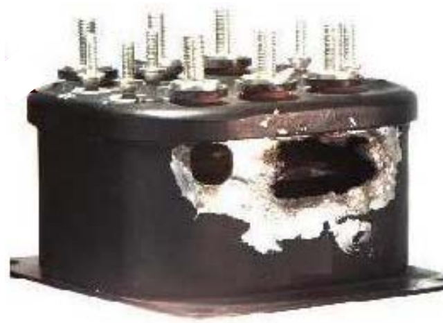
Figure 2.2 Arcing failure caused by tin whiskers [14] (Courtesy of G. Davy, Northrop Grumman Electronic Systems)
