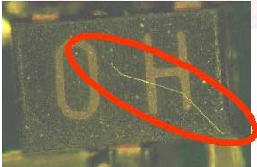
Figure 2.4 Contaminations on optics caused by whiskers [46] (Courtesy of the NASA Electronic Parts and Packaging Program)
