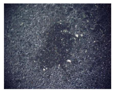
Figure 5.12: Deposit of corrosion product on mold compound after 15-day 85°C/85% RH exposure
