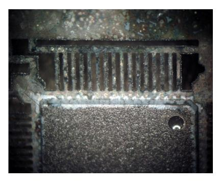
Figure 3.27 Creep corrosion over mold compound on QFP with Shinko noble pre-plated leadframe
