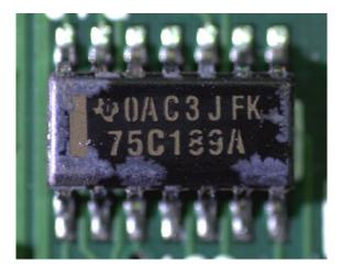
Figure 3.9 Creep corrosion on TI component over Telcordia board after 10-day test
