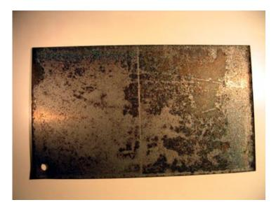
Figure 3.50 Corrosion on coupon type A after 15-day Battelle Class III test
