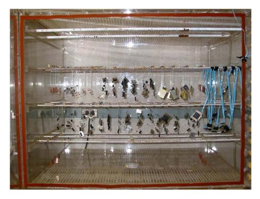
Figure 2.3 Test samples set-up for a MFG test during the study
