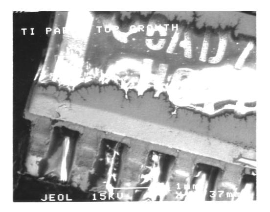
Figure 1.7 SEM overview of a failed component with creep corrosion over package
