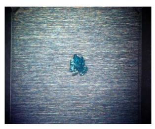
Figure 5.4: Deposit of CuCl2 on Ni/Pd/Au plated copper coupon before 85°C/85% RH exposure
