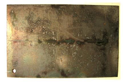
Figure 3.28 Corrosion on sample B after 10-day Telcordia Outdoor MFG test
