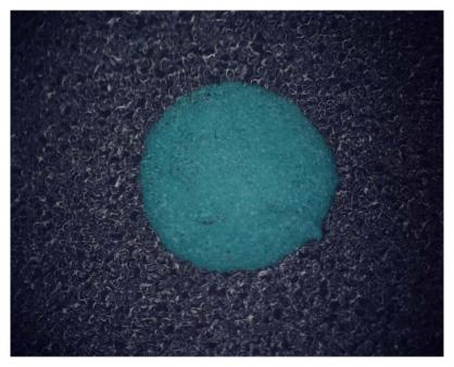
Figure 5.8: Deposit of CuCl<sub>2</sub> on mold compound surface after 15-day 85°C/85% RH exposure
