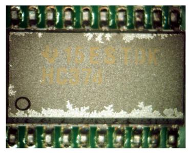
Figure 3.6 Mounted components on TI board with creep corrosion over mold compound
