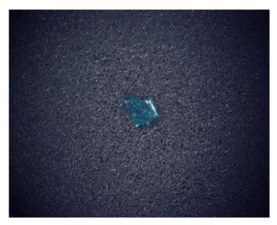
Figure 5.7: Deposit of CuCl<sub>2</sub> on mold compound surface before 85°C/85% RH exposure
