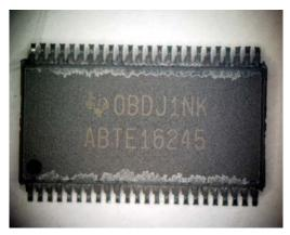
(b) Base metal: Cu (Alloy 2.4Fe/0.03Pb/0.015P/0.03Sn/0.1Zn)
