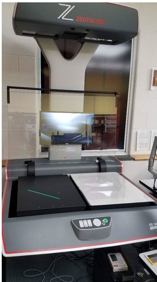
Figure 33. Newspaper issue in unopened mylar enclosure on the bed of a planetary scanner.
