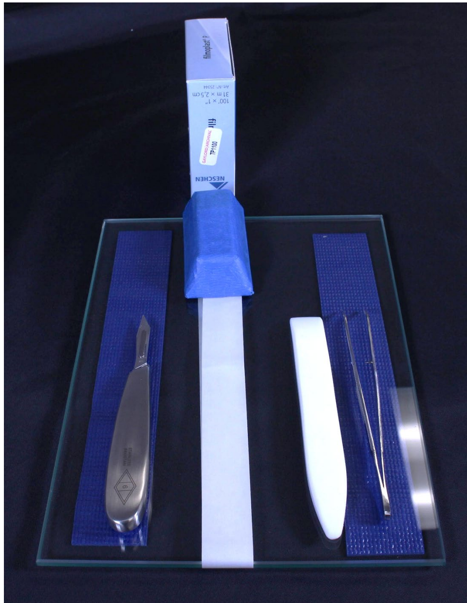
Figure 15. Setup for small repairs. From left to right: Small piece of glass with non-slip adhesive backed rubber, scalpel handle with scalpel blade, box of filmoplast™ P 90 tape, bone folder, bent-tip tweezers.
