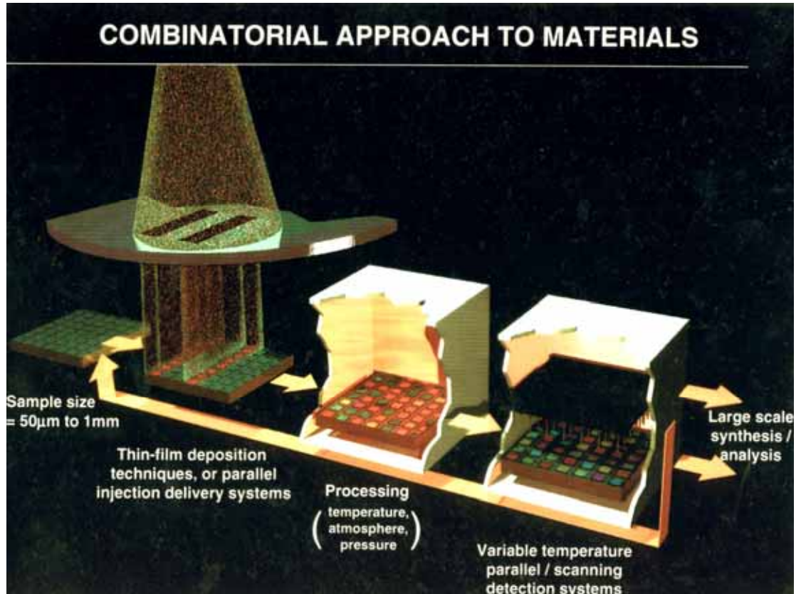
Figure 2-2: The flow diagram of a representative combinatorial thin film experiment.
