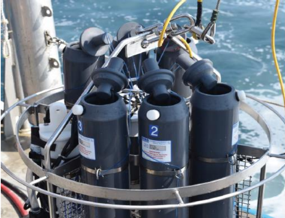
Figure 7: Photograph of Rosette with CTD and 8, 10 L Niskin bottles deployed at each sample site to measure in-situ physical parameters and collect discrete water samples at the surface, chl a max and bottom depths. Photo by Max Hermanson-UMCES- IAN (used with permission).
