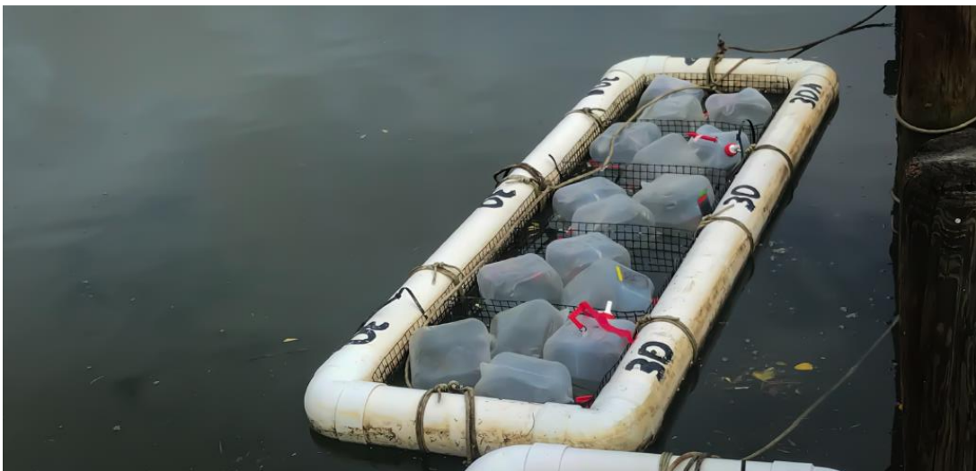
Figure 8: Taylor Floats holding bioassay cubitainers used for incubating samples at ambient light and temperature in the Horn Point Laboratory Harbor. Photo by J.M. O'Neil-UMCES- HPL (used with permission).
