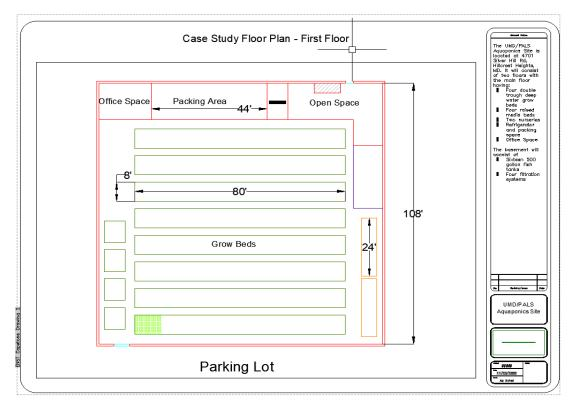
Figure 7. Main level floor plan of the case study site with the Aquaponic Source system
