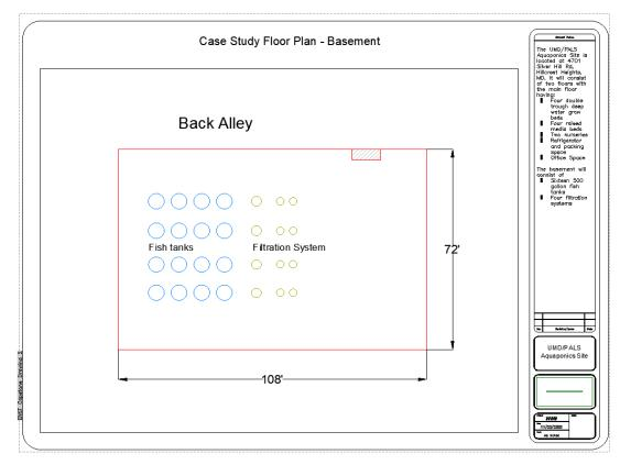
Figure 8. Basement level floor plan of the case study site with the Aquaponic Source system
