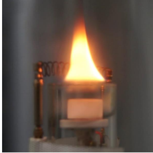
Figure 2.6: MFC test with the axisymmetric diffusion flame present at the required position i.e. the lip of the crucible housing the pyrolyzer coil
