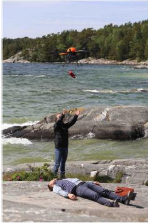
Figure 6. Drone dropping AED in simulated cardiac arrest rescue (adapted from [63]).
