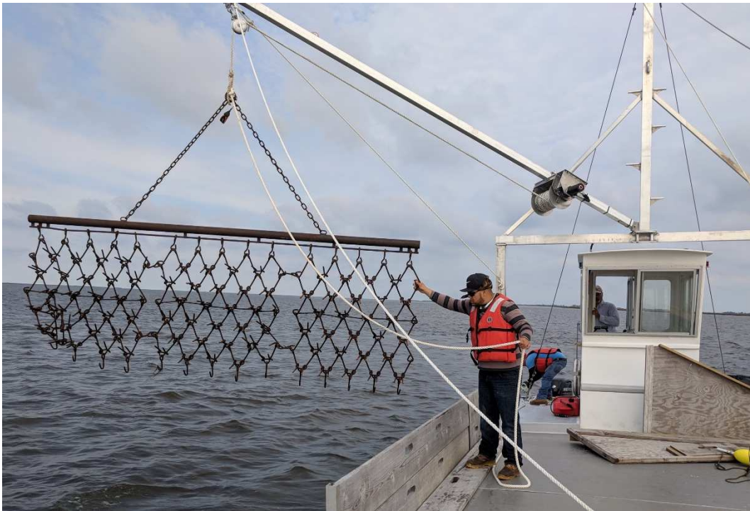
Figure 8. The harrow suspended from a vessel by a davit and winch.
