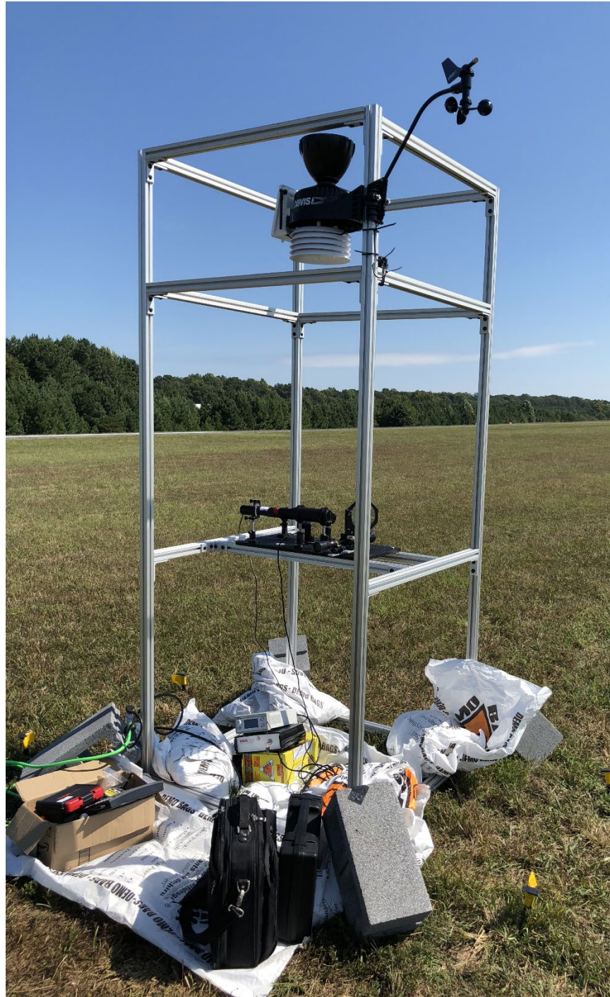
Figure 4-16: Overall view of the MAT transmitter rack. Note that vibrational stabilization is applied using both sandbags and cinderblocks at the base. A weather station is attached at the top of the rack.
