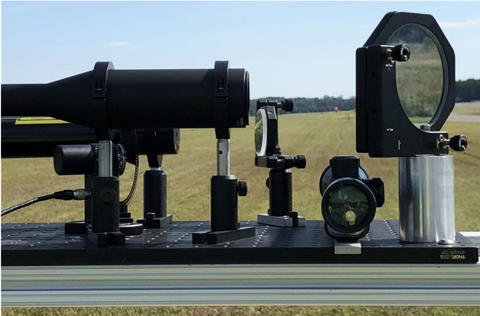
Figure 4-15: Alternative view of the MAT transmitter optical breadboard with the illuminated retroreflectors of the MAT receiver shown in the background. Note that the placement of the optical chopping wheel is shown more clearly in this figure.
