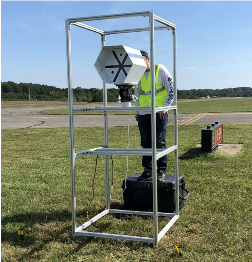
Figure 4-17: MAT receiver placed upon gimbal mount within structural framing rack and the operator shown during alignment. Note that the operator is standing upon a weatherized pelican case housing the logging computer for the MAT receiver.
