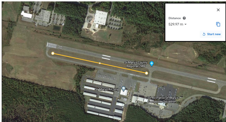
Figure 4-13: Approximate location of the Southern Maryland optical propagation path shown in within the St. Mary's County Airport complex light orange within the St. Mary's County Regional Airport complex. The MAT transmitter was in place on the east side, and the MAT receiver to the west.
