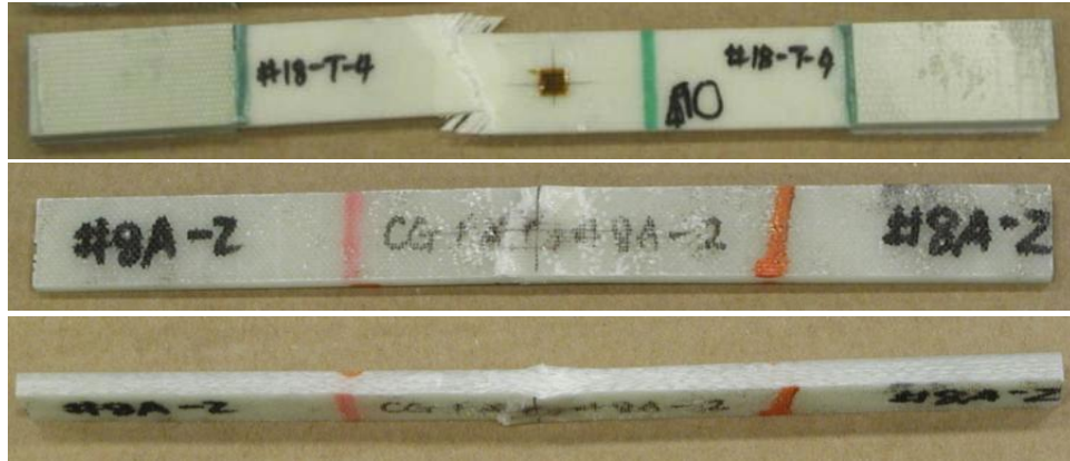
Figure 4-29. Typical failure modes observed for the tabbed tensile specimen (top) and compression specimen (middle and bottom).
