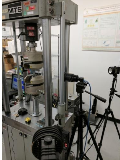
Figure 4-1 2D DIC Setup for the 4-Post 25kN MTS Frame for Round One.
