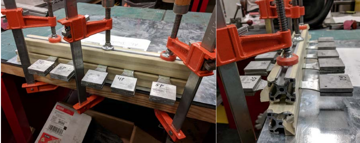
Figure 5-3 Small scale composite patch bonding jig configuration.
