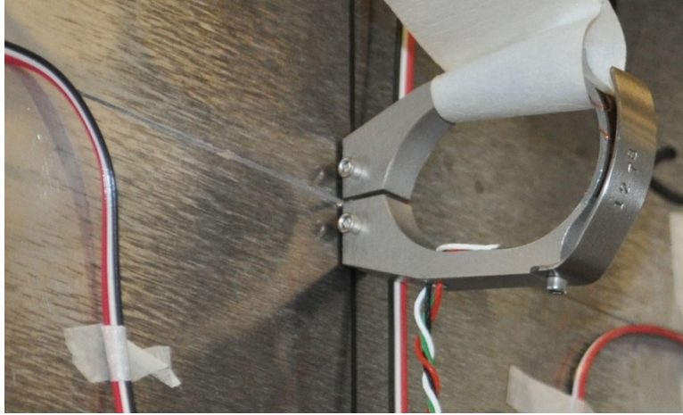
Figure 5-12: Ring gauge mounted in machined notch of specimen.
