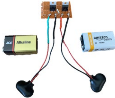
Figure 30: 9V batteries with linear regulators on perfboard
