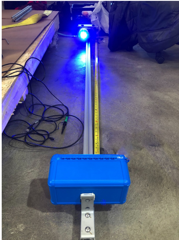
Figure 44: Photo of the rig used for underwater testing
