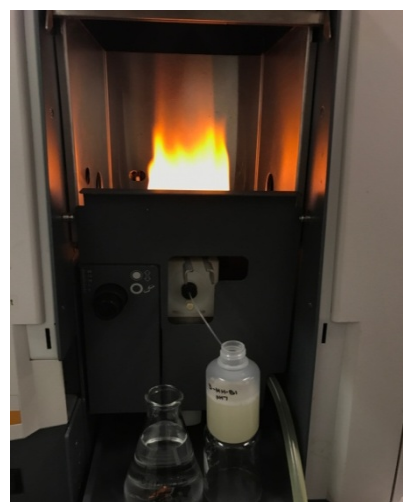
Fig. 13 - Testing with Atomic Absorption Spectrometer
