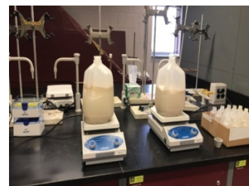
Fig. 12 - Pre-Treatment with Moringa (2-Stage Filtration)
