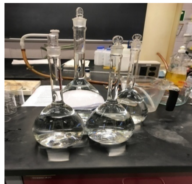
Fig. 9 - Preparation of Pb water
