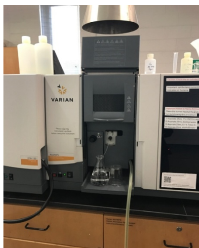
Fig. 13 - Testing with Atomic Absorption Spectrometer
