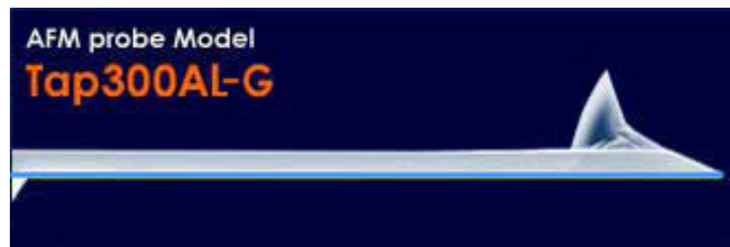
Figure 2-1 Micrograph of the cantilever tips employed for our AFM analysis. https://www.tedpella.com/probes_html/bstap300.jpg
