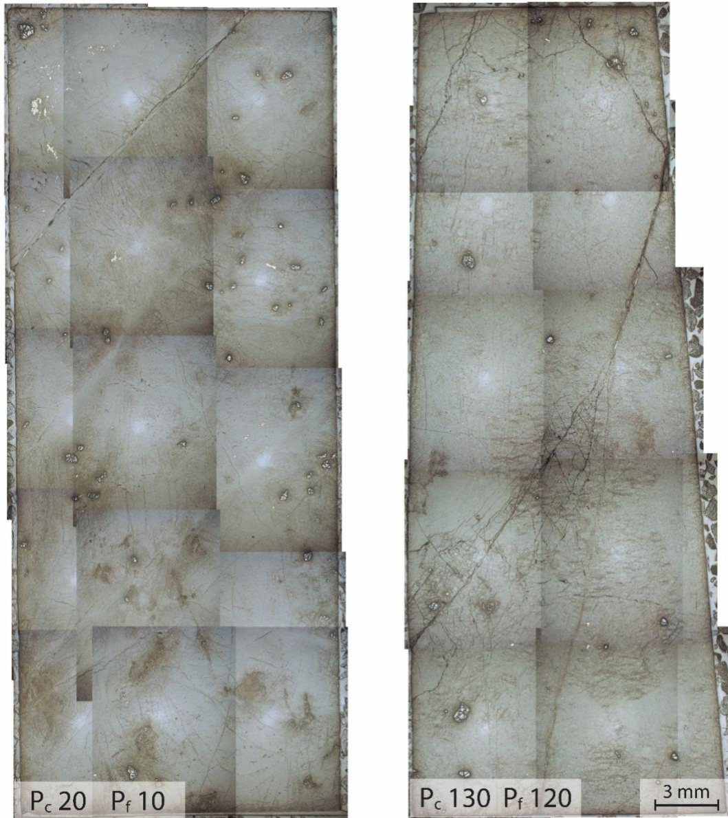
Figure 5.10: Reflected light image of microstructures of fractured Oman Dunite deformed at an effective pressure of 10 MPa and under low (10 MPa) and high (120 MPa) pore fluid pressures.
