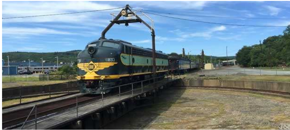
Figure 20. Restored Erie Turntable Source: Roadside America, https://www.roadsideamerica.com/tip/51933
