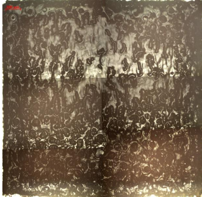
Fig. 104. non-wetted and good wetted area of PSA-substrate interface
