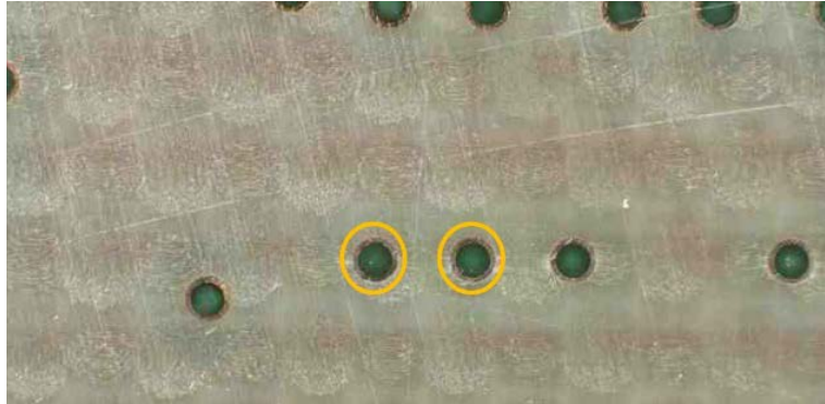
Figure 48 Bottom side (microprocessor side) view of PCB during preparation for planar sectioning. Copper layer #4 was removed to allow backside lighting. This exposed suspect vias RST_DRV and CKP+ for measurement of the drill size and via spacing.
