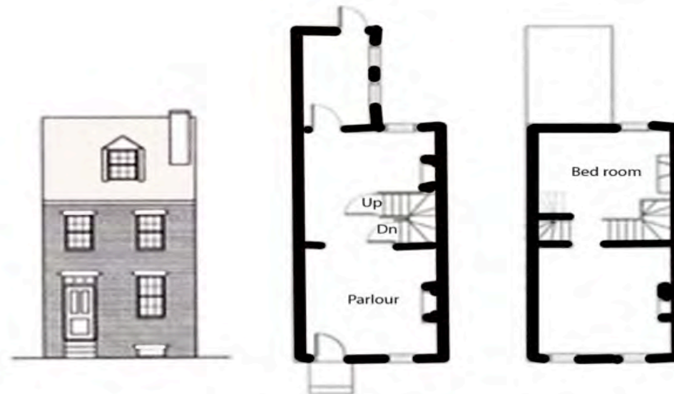
Figure 2: Floor plans and elevation of two bay wide and two rooms deep houses. (Sketch courtesy Ridhima Mehrotra)
