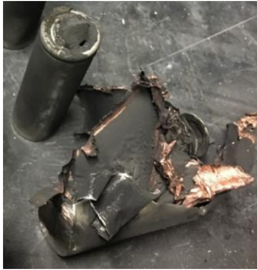
Figure 4.4: Photograph of a failed ruptured cell (bottom right) compared with a failed non-ruptured cell (top left).
