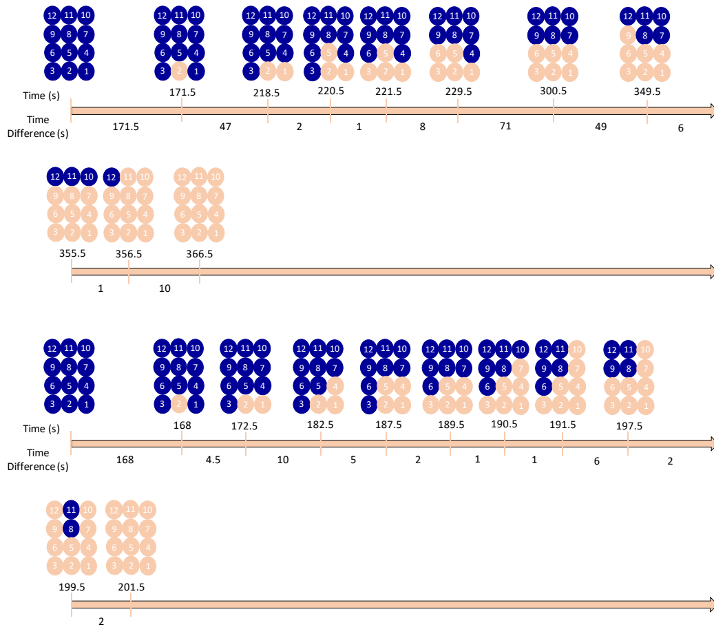
Figure 4.1: Thermal runaway propagation diagrams for example tests from the 12 cell, 100% SOC tests in N 2 (top two rows) and air (bottom two rows). Dark circles represent sound cells and light circles represent cells that have undergone thermal runaway.
