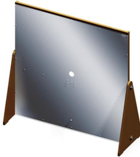
Figure 5.4. ESD calibration setup according to the IEC 61000-4-2, ESD gun is injected into the center of the plane which is a current target
