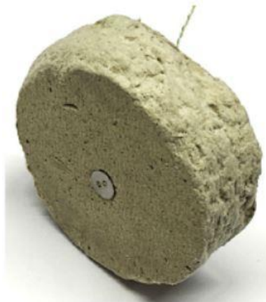
Figure 20- Real assembled thin skin calorimeter - Extracted from [20]
