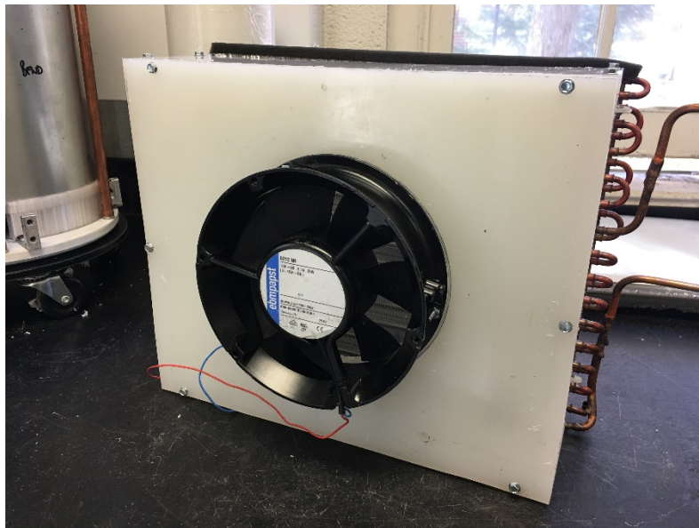
Figure 6: Heat Exchanger with 24V DC Fan
