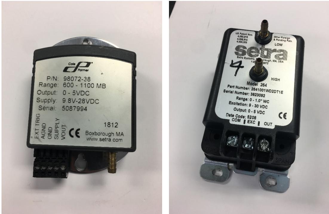
Figure 8: Air-side Barometric and Differential Pressure Transducers
