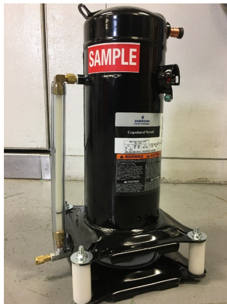
Figure 31: The Scroll Compressor with a Sight Tube
