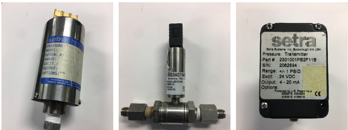
Figure 7: Refrigerant-side Absolute and Differential Pressure Transducers
