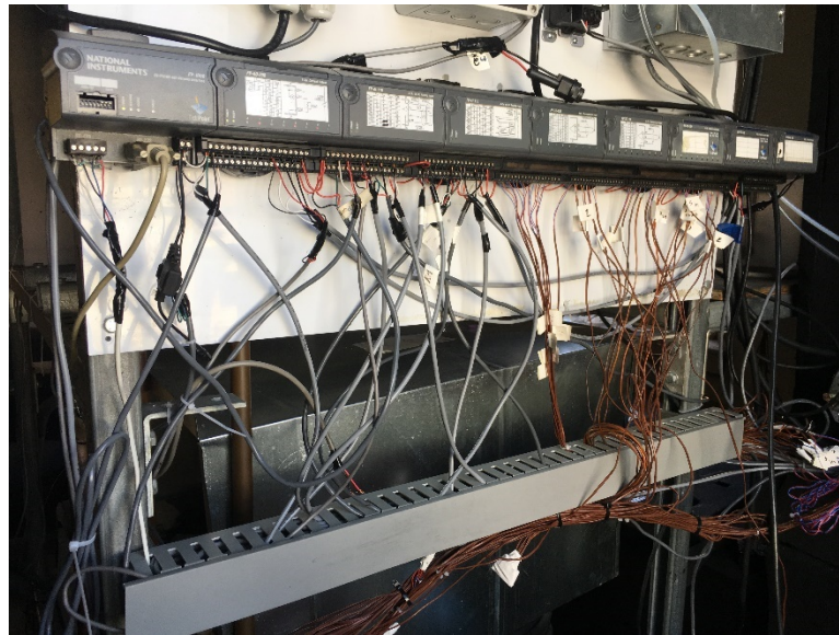
Figure 17: NI Data Acquisition Modules of the Code Tester
