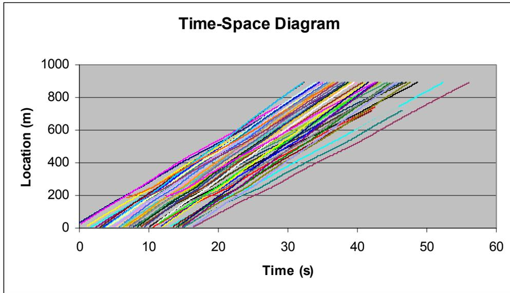
**Figure 4.3: Time-Space Diagram of the First 50 Vehicles Entering the Study Area**
