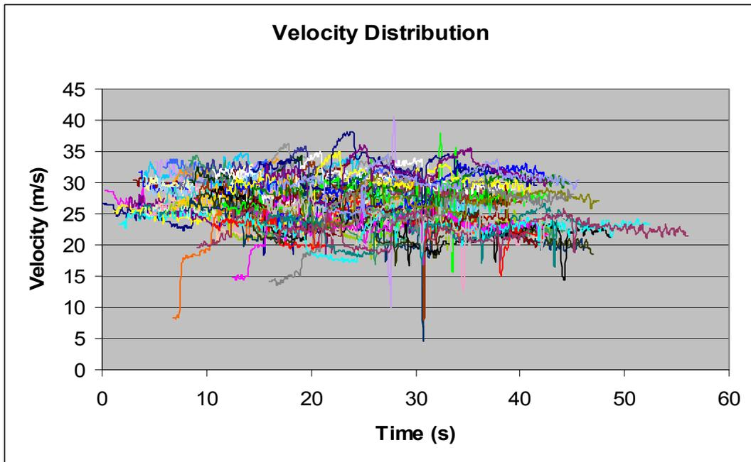
**Figure 4.4: Velocity Distribution of the First 50 Vehicles Entering the Study Area**
