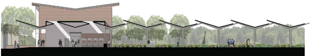
Figure 89: Section through station canopy and platform, Source by Author
