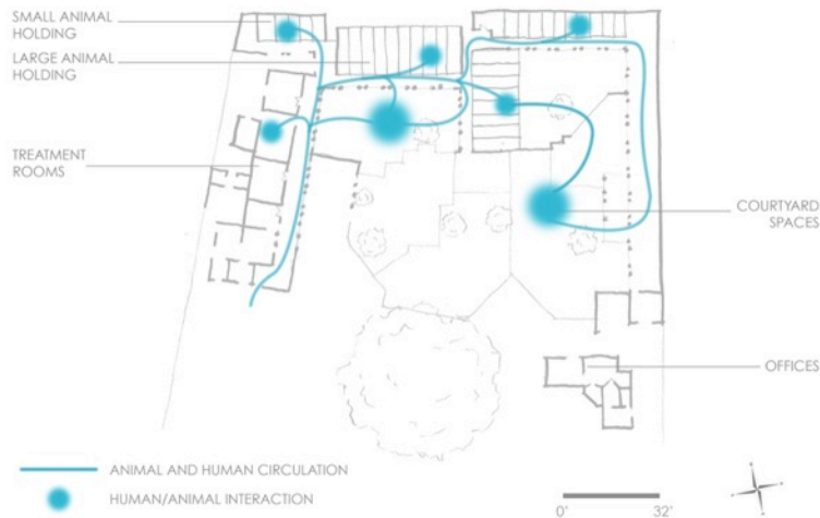
Figure 26: Sequence of circulation and human/animal interaction for employees and animals Source: Author
