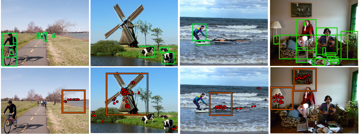
Figure 3.2: SNIPER negative chip selection. First row: the image and the ground-truth boxes. Bottom row: negative proposals not covered in positive chips (represented by red circles located at the center of each proposal for the clarity) and the generated negative chips based on the proposals (represented by orange rectangles).
