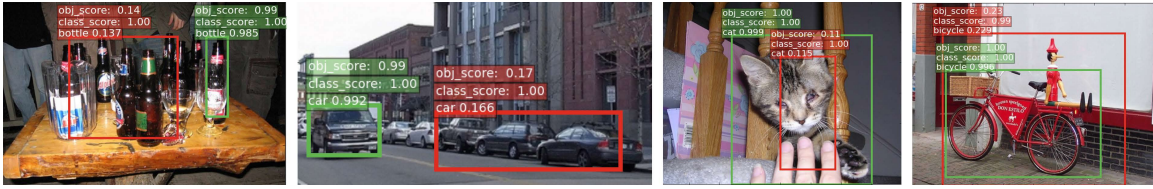
Figure 4.4: The objectness, classification and final detection scores against various transformations such as combinations of scaling and translation are shown. These scores are generated by forward propagating an ideal bounding-box RoI (in green) and a transformed bounding-box RoI (in red) through the R-FCN (objectness) and classification branch of the network. The selectiveness of the detector in terms of objectness is clearly visible against the various transformations that lead to poor detection.
