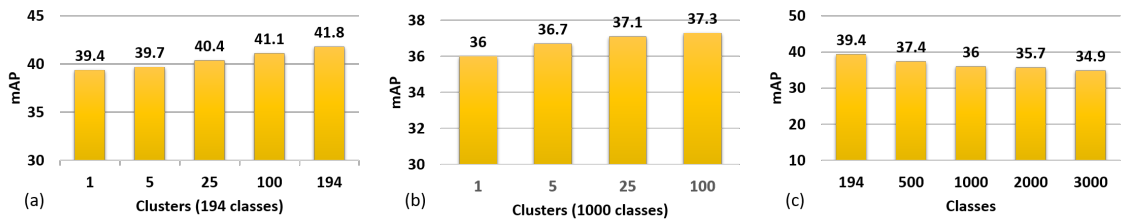
Figure 4.3: The mAP on the 194 classes in the ImageNet detection set is shown as we vary the number of clusters (super-classes). This is shown for 194 class and 1000 class detectors. We also plot the mAP for different number of classes for an objectness based detector.
