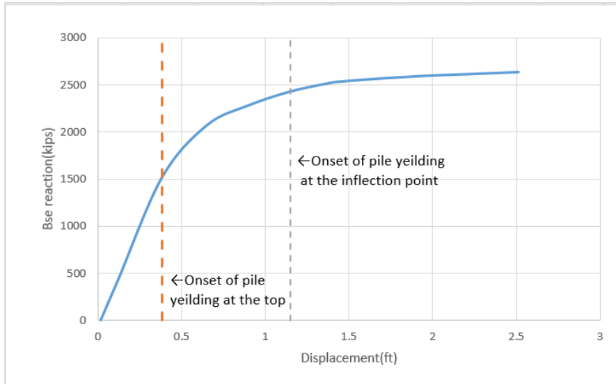
Figure 4.15-Case2 x-direction pushover curve with the mark of hinges yielding
