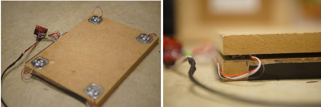
Figure 15. Weight plate showing button load cells (Left) and upper plate installed (Right)
