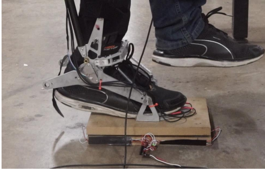
Figure 17. Testing FSRs integrated onto exoskeleton
