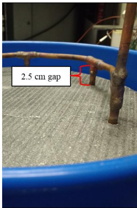
Gap before PCM backfill and cycle test
