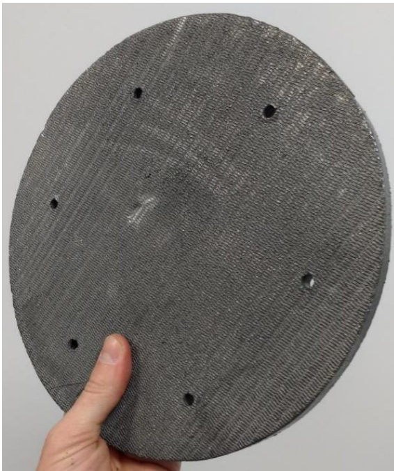
Single 25.4 cm dia. graphite-enhanced PCM disk
