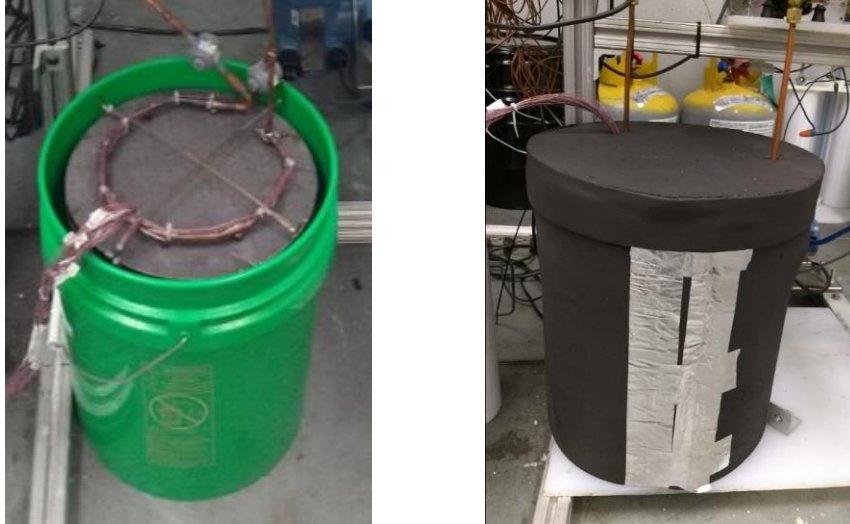
Figure 82: Different level of insulation on the graphite-enhanced PCMHX (left) and the copper-enhanced PCMHX (right)
