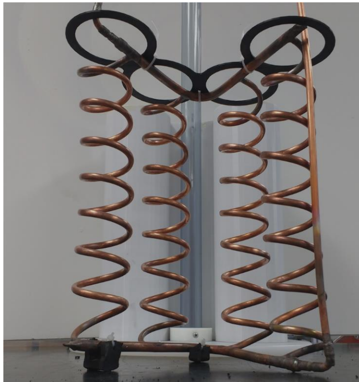
Figure 13: PCMHX Version 1: Non-enhanced PCMHX
