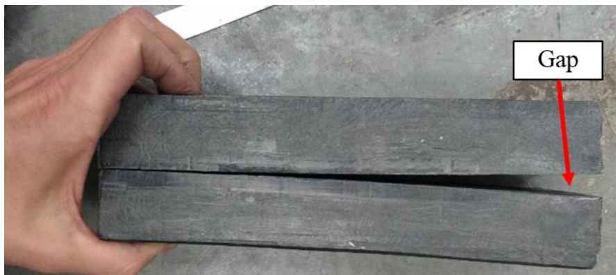
Figure 53: Warpage in the graphite blocks after post-processing
