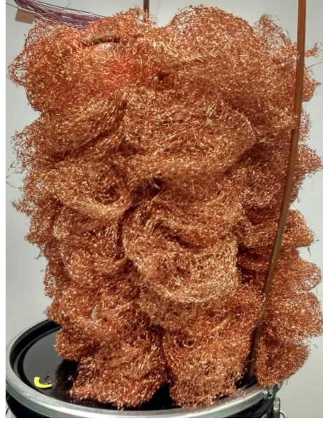
(b) PCMHEX with copper mesh
