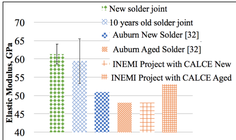
Figure 7 Elastic Modulus of solder joints from our testing and literature reports
