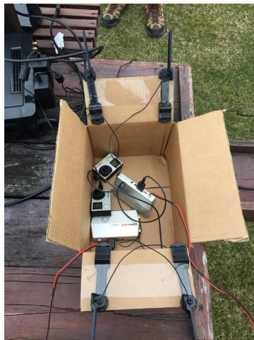
Figure 34: Initial Connex communication test mobile UAV portion Connex setup.
