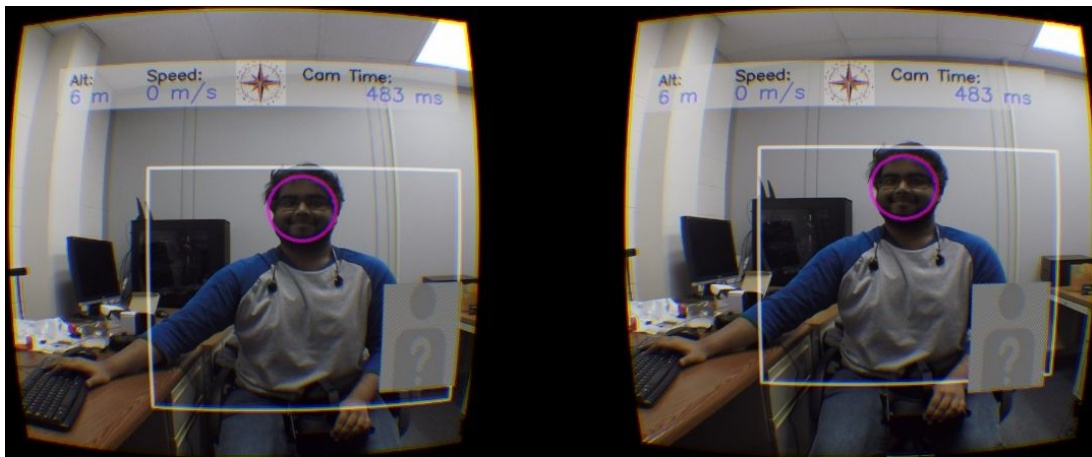
Figure 21: Augmented overlays and facial recognition on stereo camera system.
