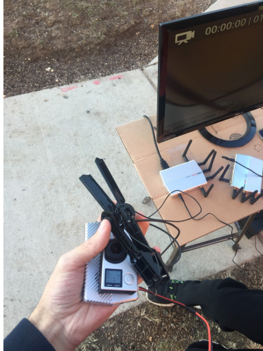
Figure 32: Initial Connex communication test materials including: a GoPro, 2 Connex transmitters and antenna located in the hand, and 2 Connex receivers and a monitor located on the table.
