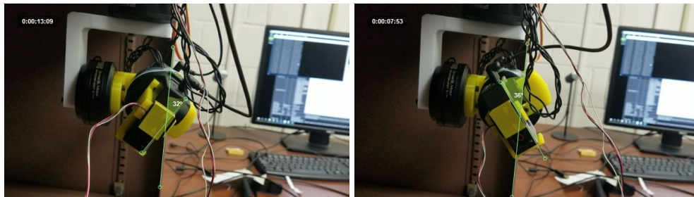
Figure 31: Pitch axis control of custom gimbal at 36° (left) / -32° (right).
