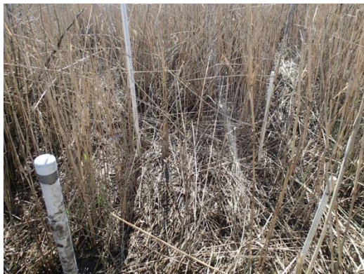
Figure B.3.5. Image of continuous data logger well, installed at God's Grace.
