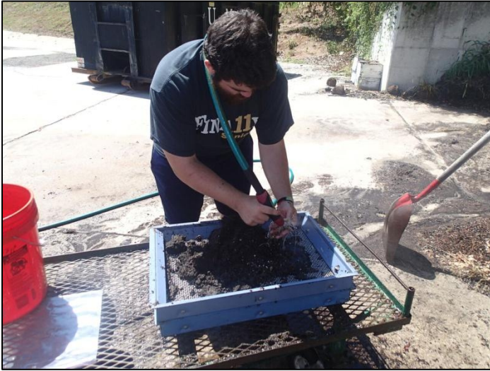
Figure B.2.21. Photograph of root washing. Growth media was washed away from belowground parts using a garden hose and a 5 mm mesh screen.
