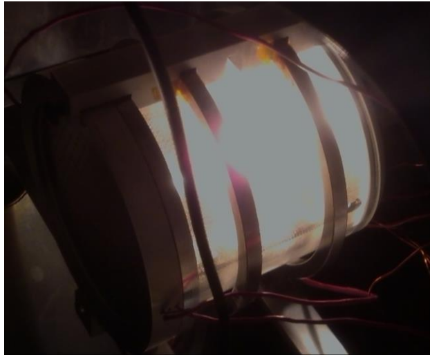
Fig. 112: SPPL-1 First Plasma Ignition
