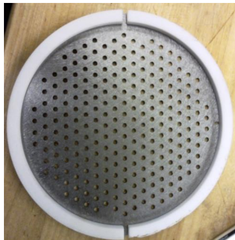
Fig. 110: SPPL-1 Optics Grids w/Alumina spacers
