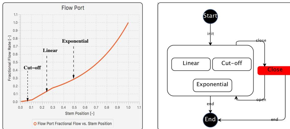
Figure 6.1: Hybrid behavior of a valve.
