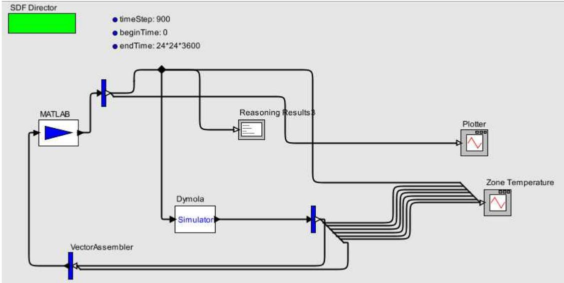
Figure 5.4: BCVTB framework DTS-based MPC and Modelica simulation model.
