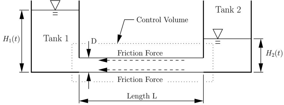
Figure A.3: Summary of forces acting on a pipe element connecting two tanks.
