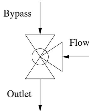
Figure 2.10: Schematic for a three-port valve.
