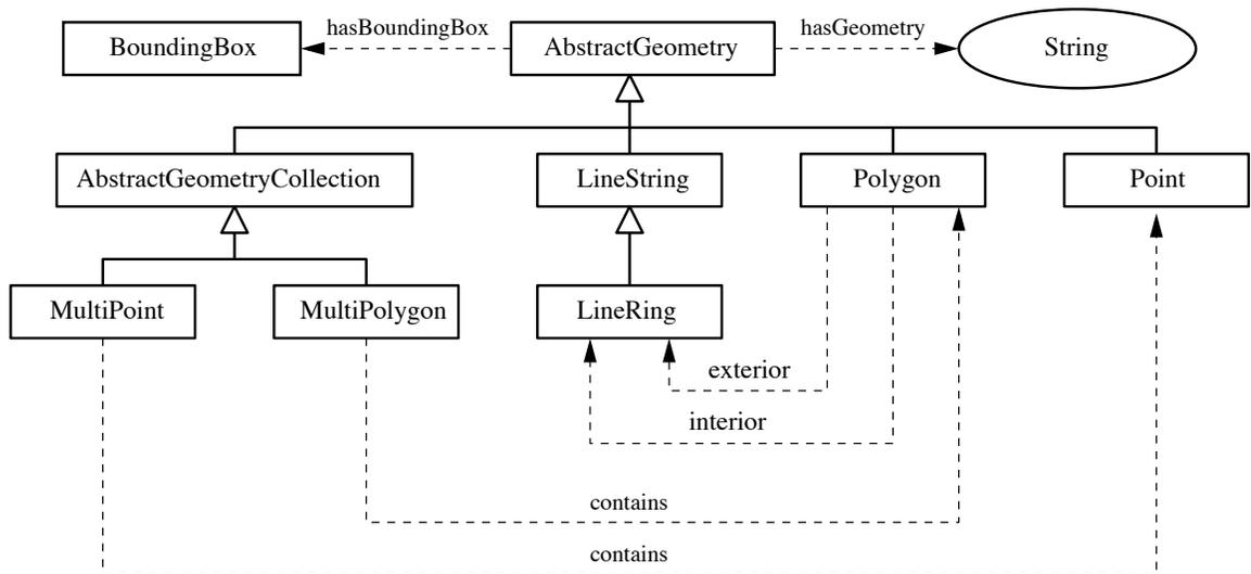
Figure 4.5: Abbreviated representation of spatial (geometry) ontology and associated data and object properties.
