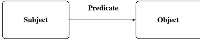
Figure 2.2: Example of RDF triple where node A is a subject, "predicate" is a verb, and node B is an object.
