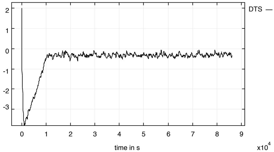
Figure 5.6: Dynamic thermal sensation model – Acceptable range is  $-0.5 < DTS < 0.5$
