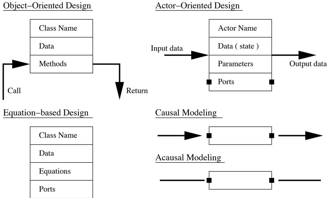
Figure 3.4: Five approaches to system/model development: (1) object-oriented, (2) actor-based, (3) equation-based, (4) causal modeling, and (5) acausal modeling (Adapted from Lee [83]).
