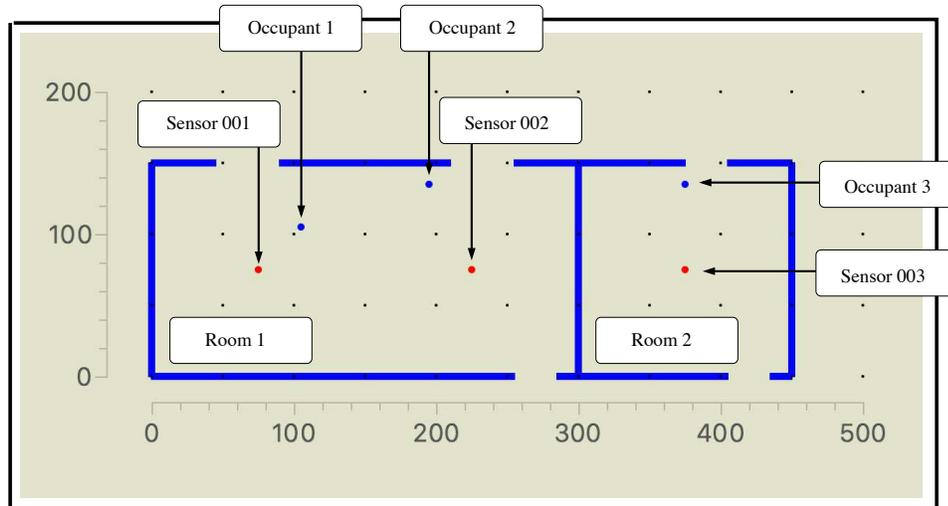
Figure 5.16: Plan view of two-room building architecture, sensors, and building occupants.
