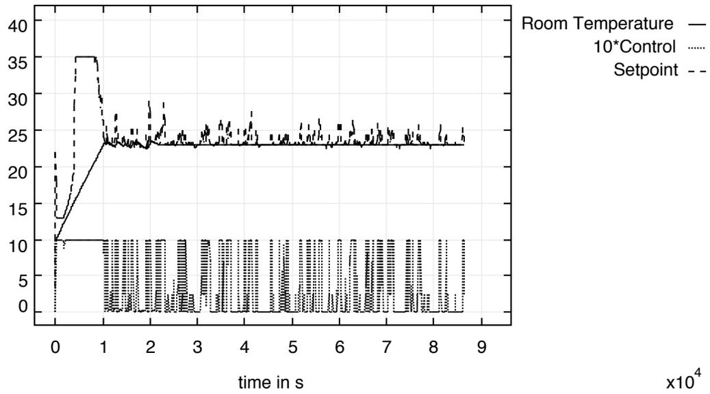
Figure 5.5: Setpoint, room temperature, and control signal.
