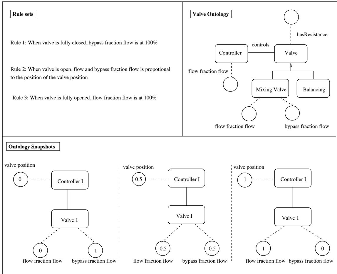
Figure 2.9: Schematic for a valve ontology and rules.
