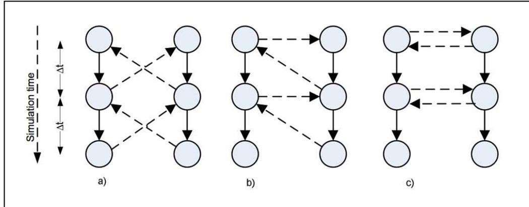
Figure 3.5: Three strategies of data exchange in energy co-simulation: (1) strong coupling of time-dependent states, (2) loose coupling with sequential simulator execution, and (3) loose coupling with parallel simulator execution.
