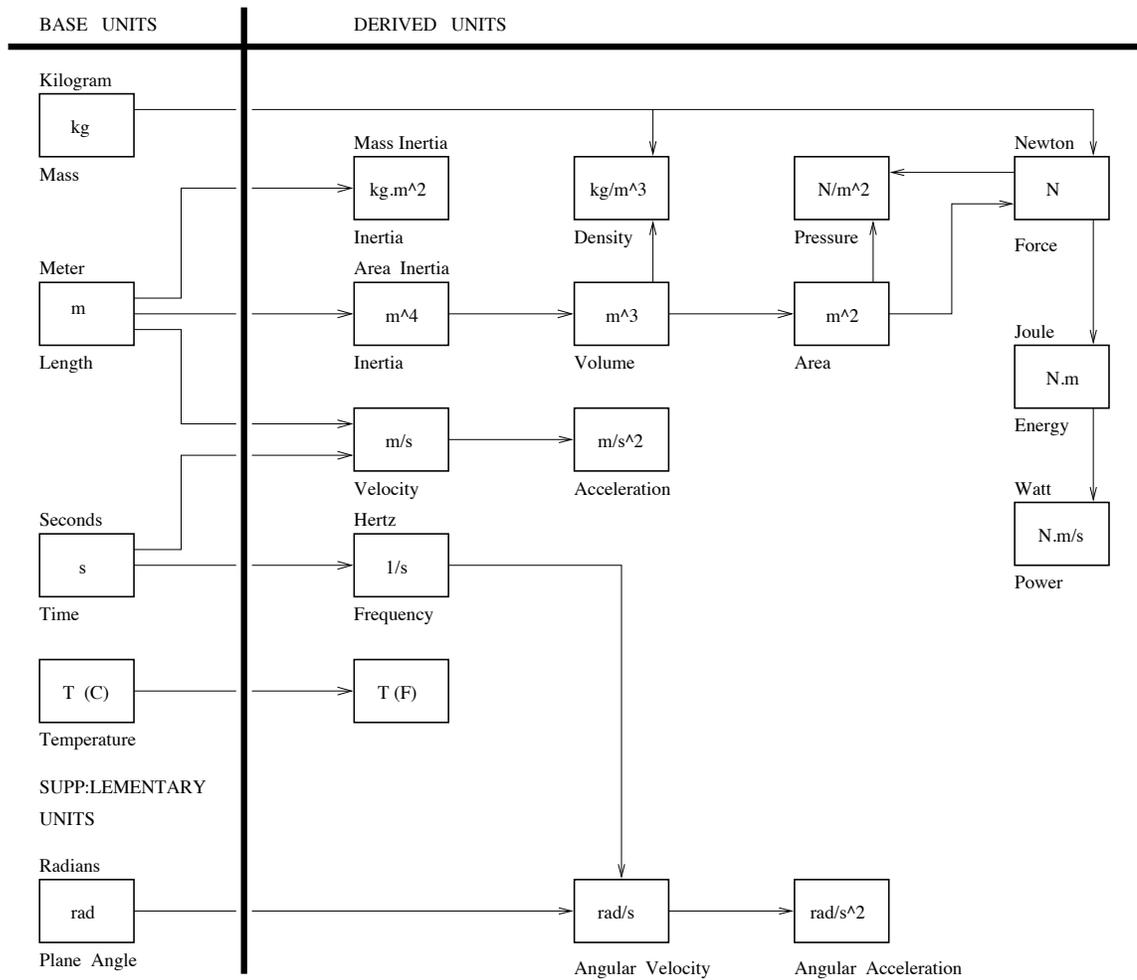
Figure A.1: Primary base and derived units commonly found in engineering mechanics.
