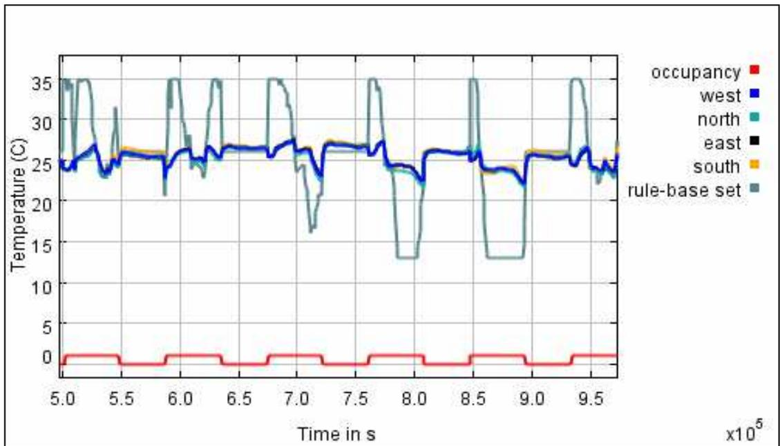
Figure 5.9: Profiles of room occupancy, rule-based setpoint, and temperature versus time (sec) for Control Case 1.
