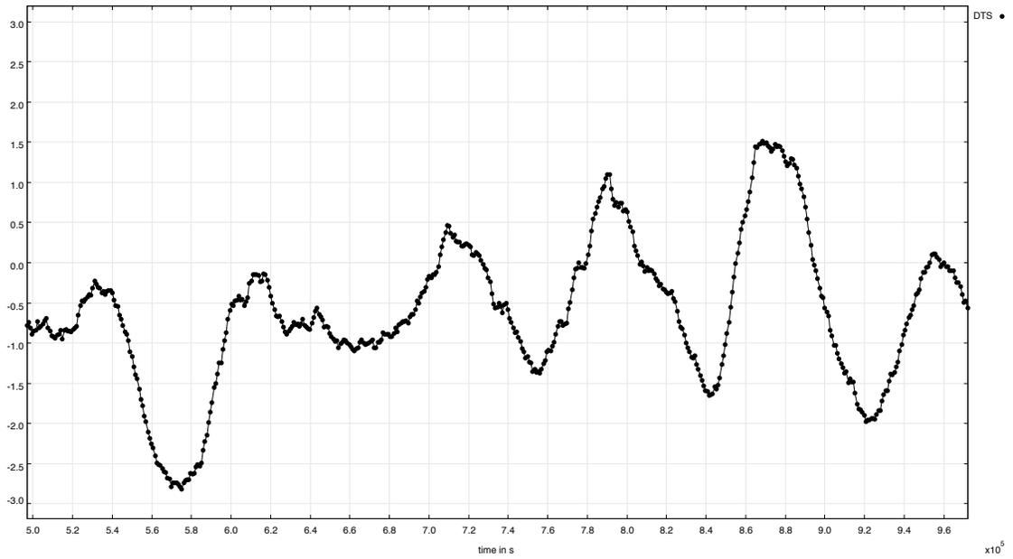
Figure 5.7: Dynamic thermal sensation index versus time (sec) for Control Case 1.
