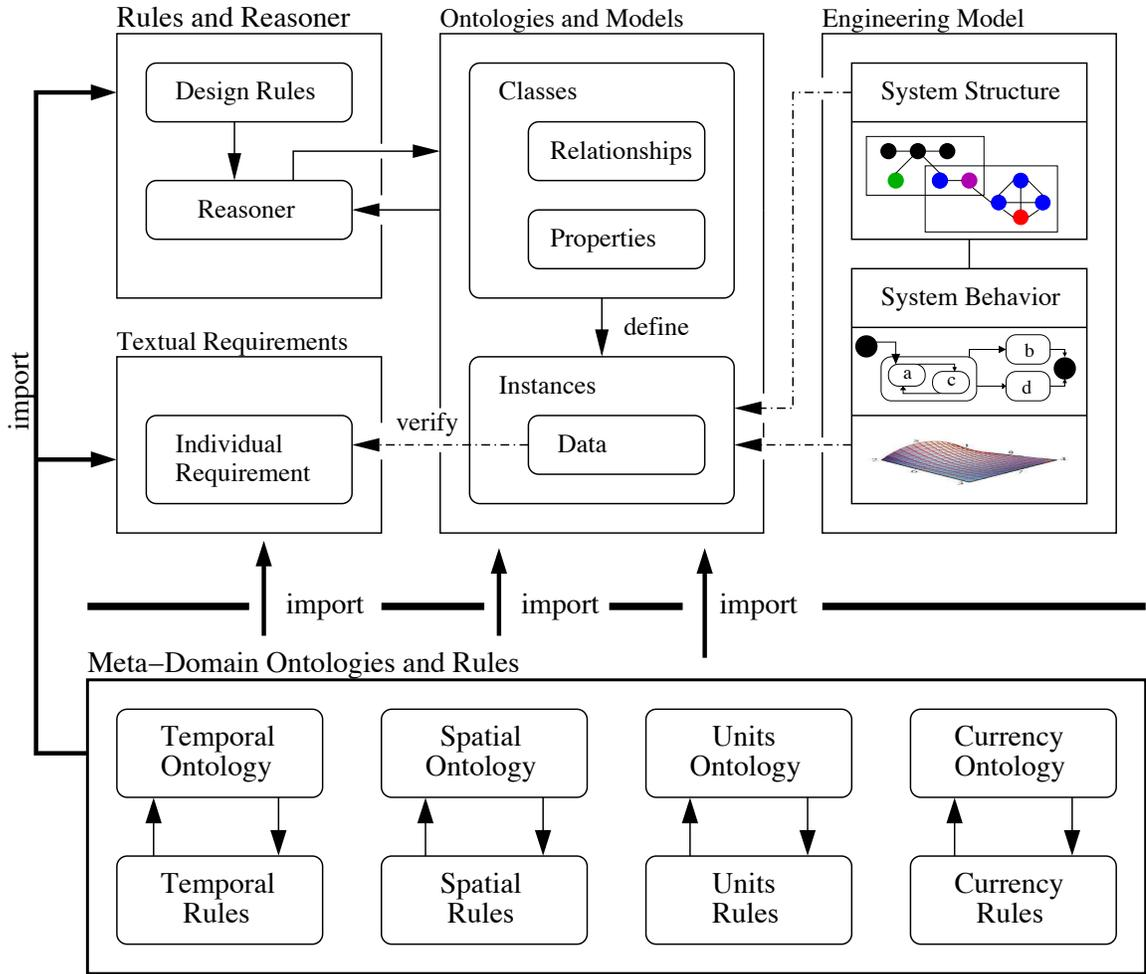
Figure 1.1: Framework for implementation of semantic models using ontologies, rules and reasoning mechanisms.
