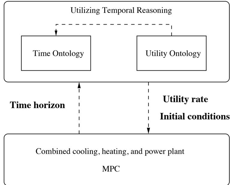
Figure 5.12: Multi-level control structure for HVAC systems.
