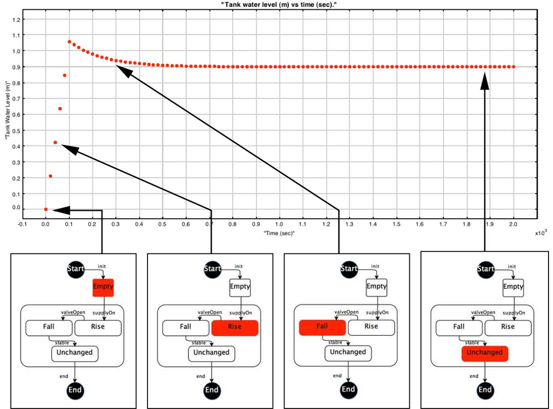
Figure A.7: Time-history response for a tank having a water supply and shut-off valve. Upper plot: tank water level (m) versus time (sec). Lower plot: discrete statechart behaviors at various points in the time-history response.
