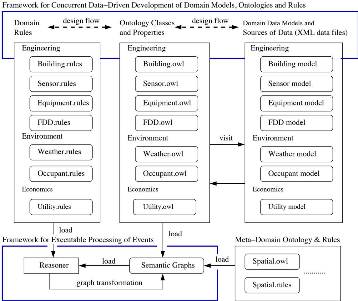
Figure 1.2: Contribution 1: Systems architecture supporting: (1) concurrent data-driven development of domain models, ontologies and rules, and (2) executable processing of events.
