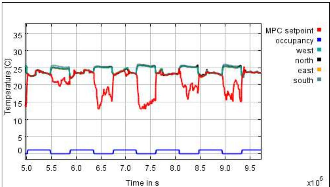
Figure 5.10: Profiles of room occupancy, MPC setpoint, and temperature versus time (sec) for Control Case 2.
