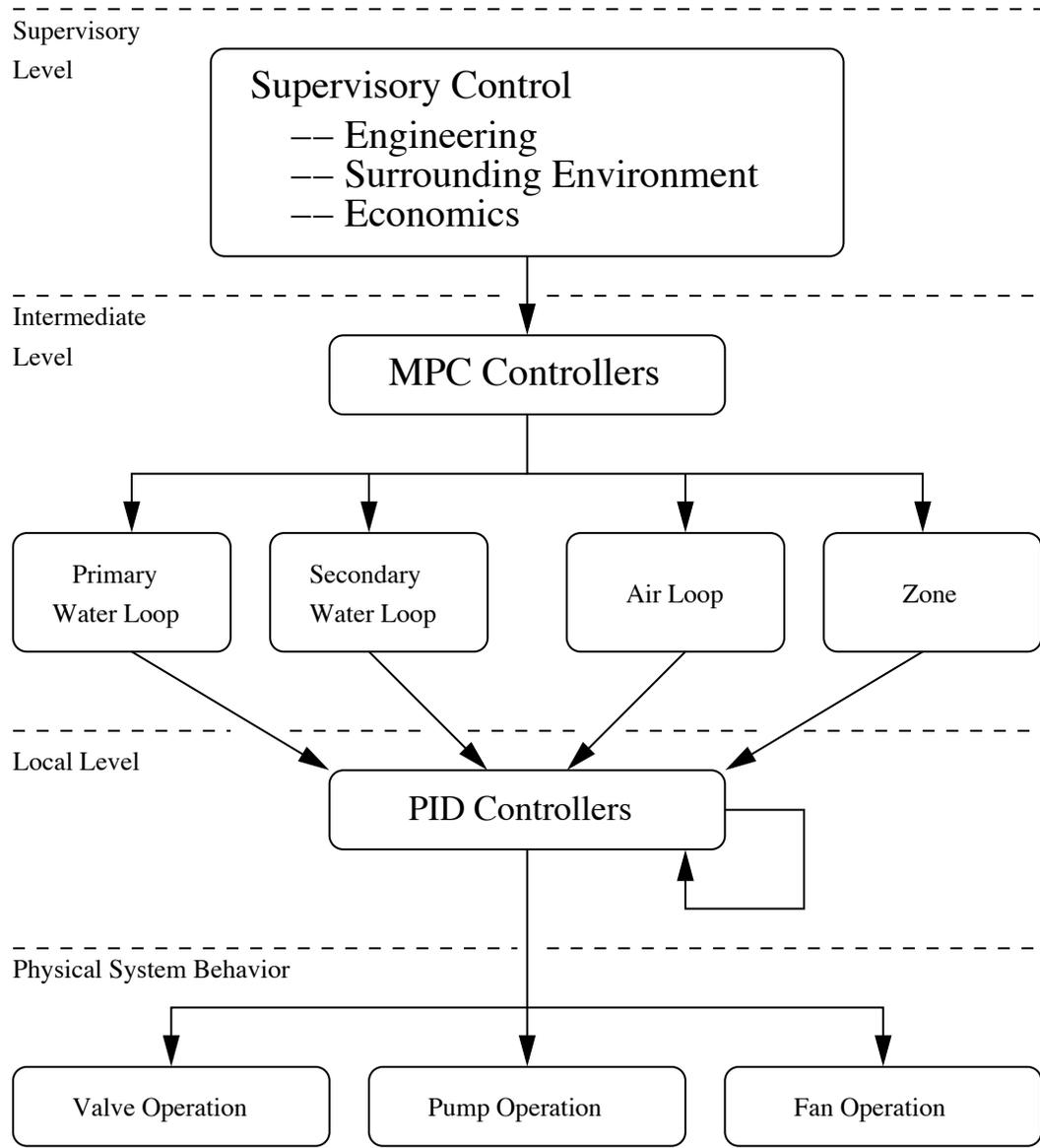
Figure 3.7: Multi-level control structure for HVAC systems.
