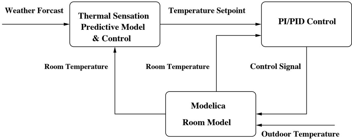
Figure 5.3: Flow diagram for data exchange in BCVTB
