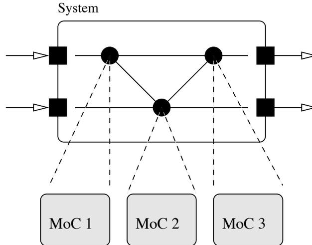
Figure 3.3: Different parts of a system are modeled with different computational models. The separate models of computation are integrated into a single framework. Models of computation can potentially include finite state machines (FSMs), communicating finite state machines (CFSMs), continuous time (ODEs), continuous time over spatial dimensions (PDEs), discrete event systems, data flow models and signal models.
