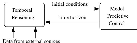
Figure 5.11: Architecture for coupled semantic/MPC HVAC system control.
