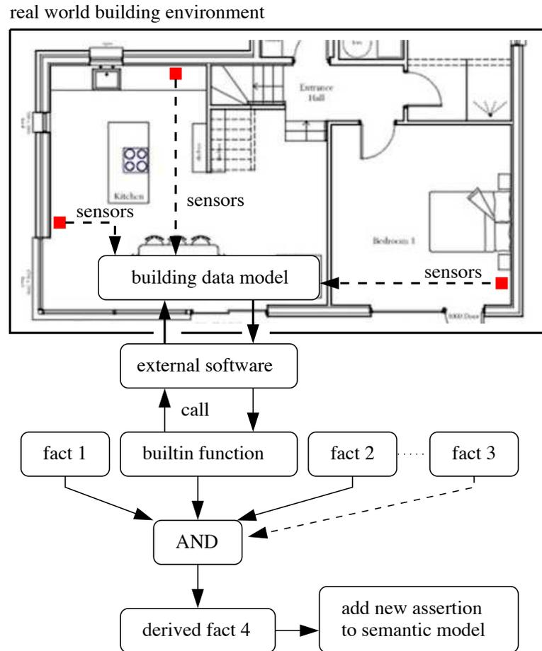
Figure 2.6: Framework for forward chaining of facts and results of builtin functions to new assertions (derived facts).
