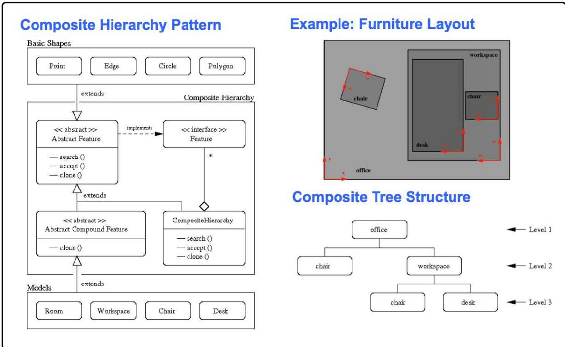
Figure 1.6: Collage of composite software design patterns and simple applications.
