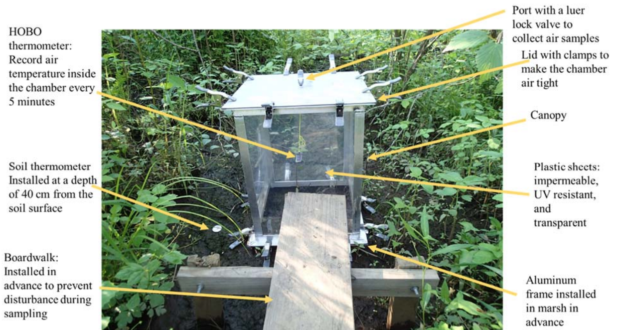
Figure C.1: Field photo showing the gas flux chamber setup.
