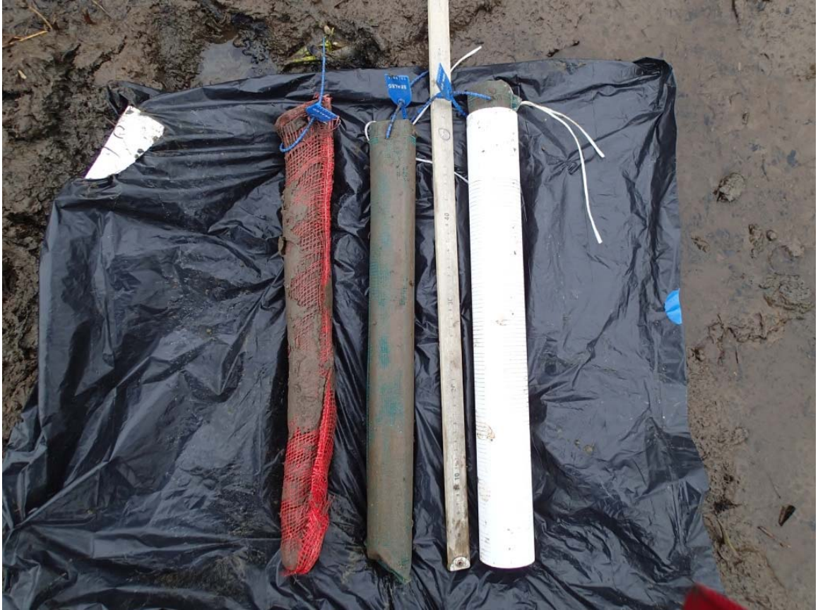
Figure 3.1: Field photo showing the three types of CARBIO. From left to right: large mesh, fine mesh, and fine mesh inside the slotted PVC. Photo credit: Andrew Baldwin.
