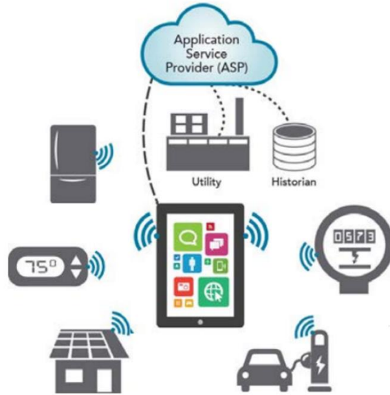
Figure 2.2: Data transfer from and to devices via VOLTTRON. Note VOLTTRON does not have a GUI. The depiction of the center tablet is for visualization purposes. Image from [32]
