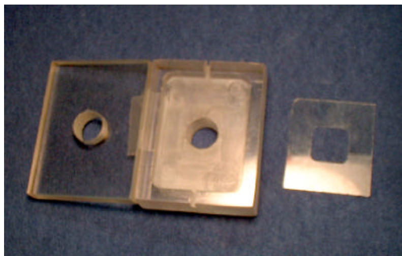
Figure 5-26 Mesopump housing and Pyrex spacer
