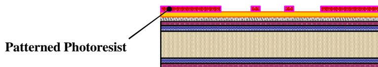
Figure 5-15 Photoresist is patterned on the wafer front side
