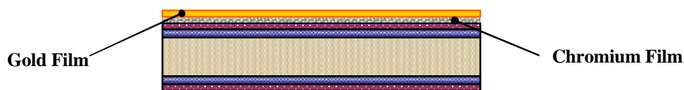
Figure 5-13 Schematic sketch of the wafer cross-section after chromium-gold deposition
